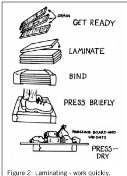
Figure 2: Laminating - work quickly, race-the-stretch
